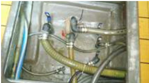
All fuel and water tanks are in good condition as can be inspected. The fuel lines, including a Racor filter are approved type and in good condition. The flex fuel line appears to be a recent upgrade. The fuel fills, vents and shut-off are in good order.
