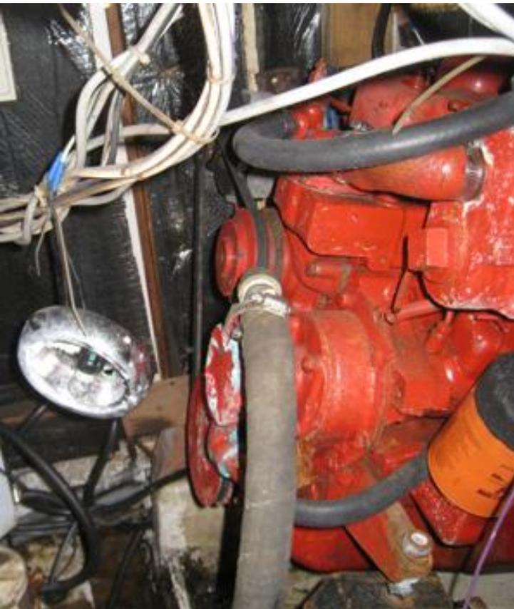
The monel shaft and related hardware are in good condition as can be inspected from the inside. The shaft log is in good shape, properly secured and clamped. The engine compartment is reasonably clean and free of any unessential gear. The fuel tank is secured and inspection was not possible. The fuel shut-off is easily accessible. The fuel feed lines and fill are in good condition and secure.
